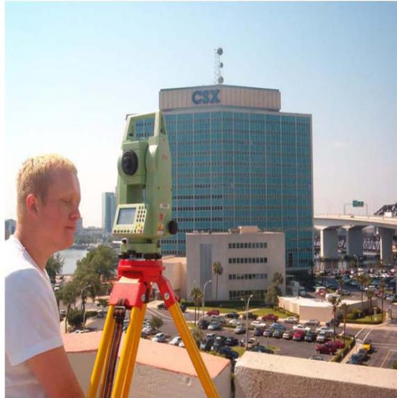
**Leica TCR-705 Reflectorless Total Station (Geodetic Services, Inc.)**
